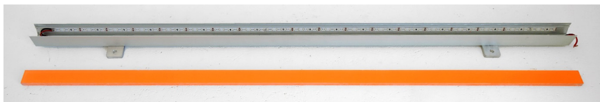
Figure 4 SCW-60 Version 1 (2018), luminaire made of an aluminium body, cyan LED strips and a red-orange remote phosphor coated on transparent polycarbonate.
